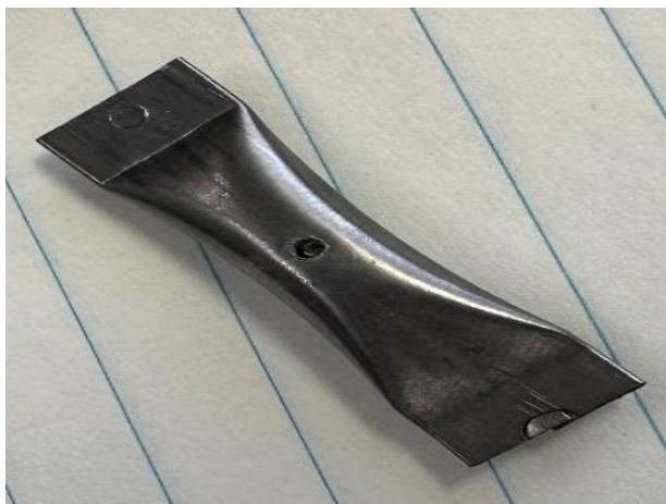
Fig. 1. Tantalum pinhole boat containing a pressed pellet of \text{Sm}_2\text{O}_3 and Zr.
